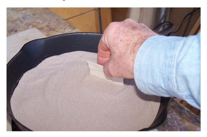
Use your piece of scrap veneer to test when the sand is hot. Just stick the veneer into the sand a bit - not all the way that it hits the bottom of the pan. When the veneer will shade in 15 to 20 seconds, the sand is hot enough. This is about what you're looking for (next picture). [Update 3/5/2012: I now expect the veneer to shade quicker, between 5 and 10 seconds.]
