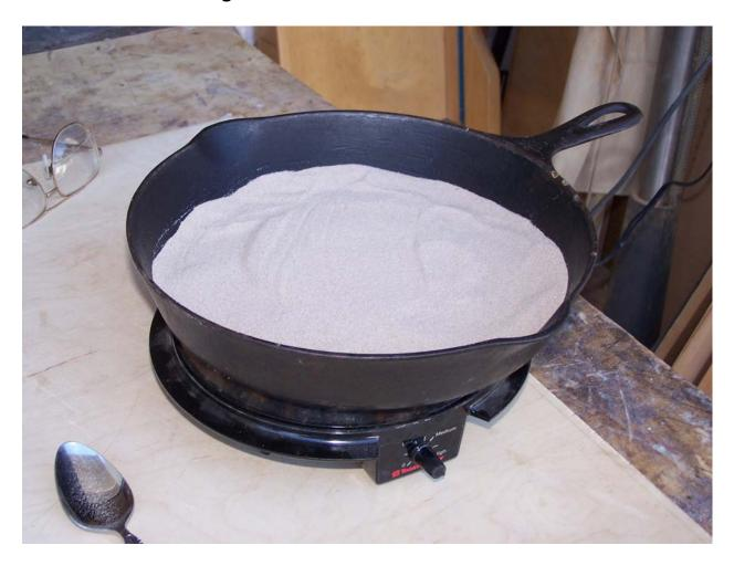
You want to smooth the top of the sand so that when you put the veneer into it, the line of shading is smooth and not "lumpy". You can use a spoon to smooth the sand out or just take a piece of scrap veneer and use that to smooth it out.
