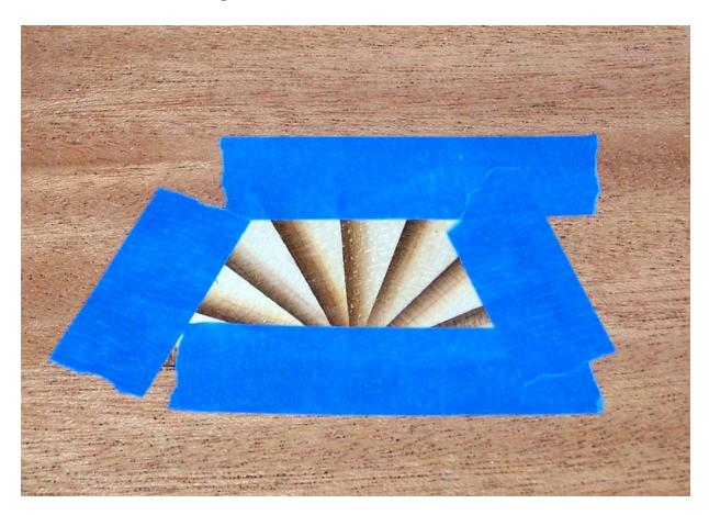
Turn the veneer over so that the show face is up and tape the fan in with veneer tape.
