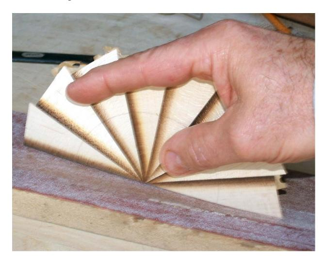
The next step determines the size of the fan. Choose a carving gouge and see where it comes to when you position it so that it will cut across a wedge. The gouge shown is a #7 gouge, 16mm wide. A wider gouge will give a larger fan while a narrower gouge will give a smaller fan. I find that a #7 gouge has a pleasing arc for the fan but you may prefer
