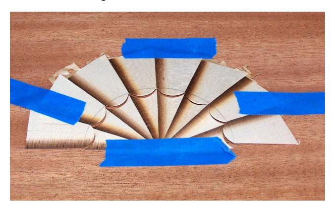
Remove the waste veneer from the fan and tape the top of the fan aligned with the cuts you just made. Cut the field veneer using the bottom of the fan as a guide. Once you complete the cut, remove the fan and snap out the waste from the field. You'll have a fan shaped hole in the field like the following.
