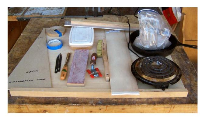
The items we have in the picture are as follows. On the left we have the 16 segment template. At the top and just to the right of the template we have the veneer tape and the blue tape. Just below that is the Japanese marking knives used for cutting the veneer, and a 16mm #7 carving gouge. Above that is the container with a sponge and water for use with the veneer tape, and a straightedge lying on the container. Below that is a sanding block, a veneer saw, and a brass
