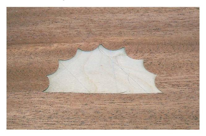
Put the fan into the cutout and tape it with blue tape.
