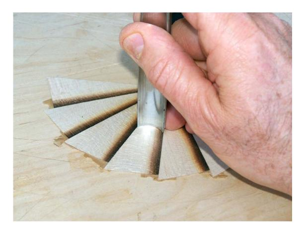
Mark the location on the fan where the gouge fits. Then take a compass and draw an arc through that mark, using the points of the fan as the center of the arc. DO NOT cut the arcs on the fan yet.
