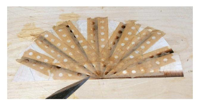
Let the tape dry well - set the piece aside for some time, and press it between two pieces of wood to keep it flat while it is drying. Once it's dry, turn the fan over and remove all the blue tape from the glue face.
