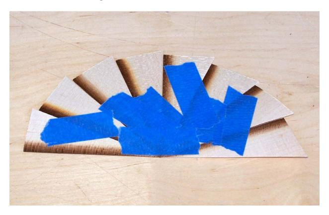
Now, turn the fan over so that the show face is up and tape the seams with veneer tape. We do not want more than four layers of veneer tape so plan your taping to minimize overlap.
